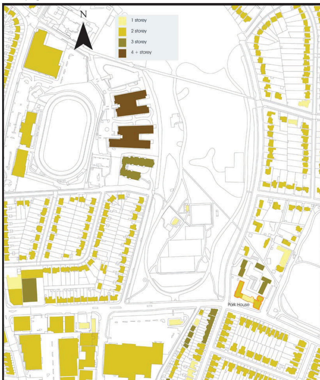
Figure 3 : Storey heights of existing buildings
